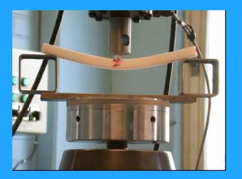
The material can easily be processed to withstand bending strains to a sufficient degree for flexible district heating pipes.
