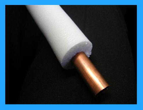
According to the present study PET foam seems to have the potential to compete successfully with cyclopentane blown PUR foam as insulating foam for district heating pipes of small dimensions at low temperatures (<100°C).
