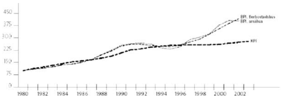
Figure 21: Development of building costs. Building price index BPI compared with consumer price index KPI (according to Swedish competition authority).
