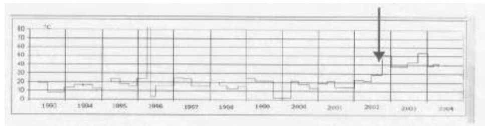
Figure 6.2-4: Substation cooling record at a shopping mall in Göteborg, Sweden.
