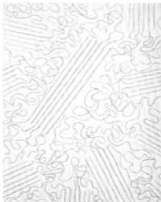
Figure 8.2: The structural arrangement of HDPE chain molecules. (Source Wirsbo, [20]).
