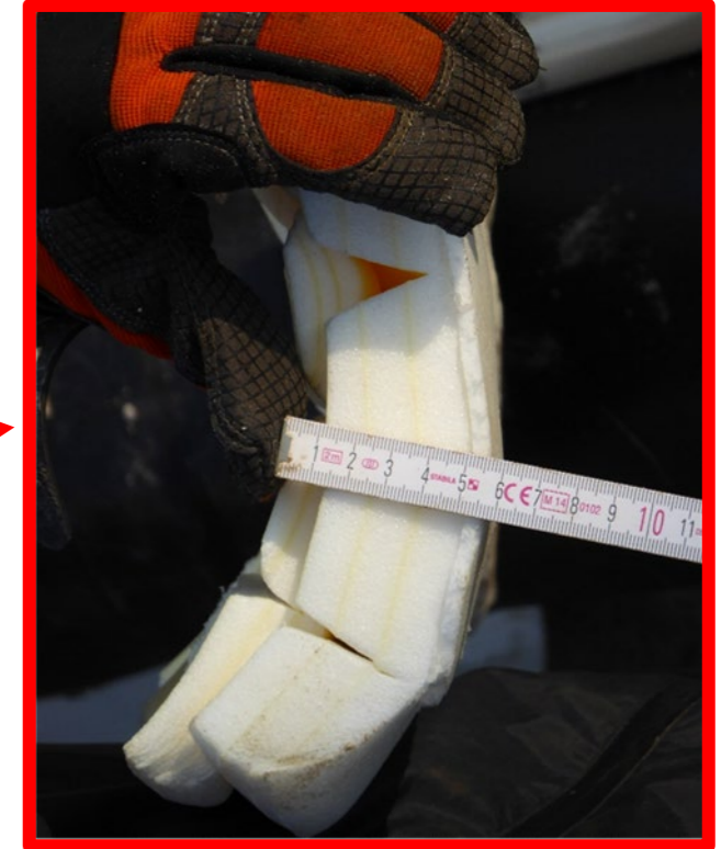
Cushions after 50 full load cycles @ AGFW research section in Chemnitz (origin 80 mm according to the design), Investigations done by IGtH Hannover & AGFW
