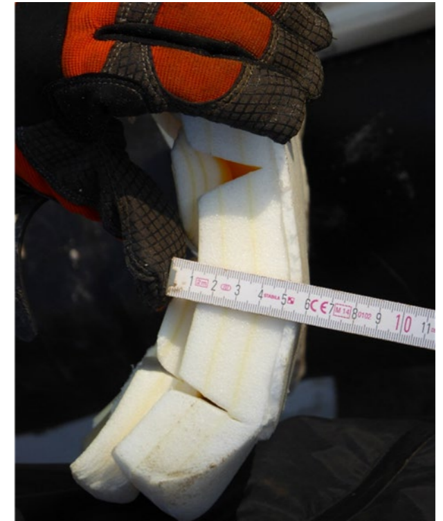
Cushions after 50 full load cycles @ AGFW researche section in Chemnitz (origin 80 mm according to the design), source: AGFW
