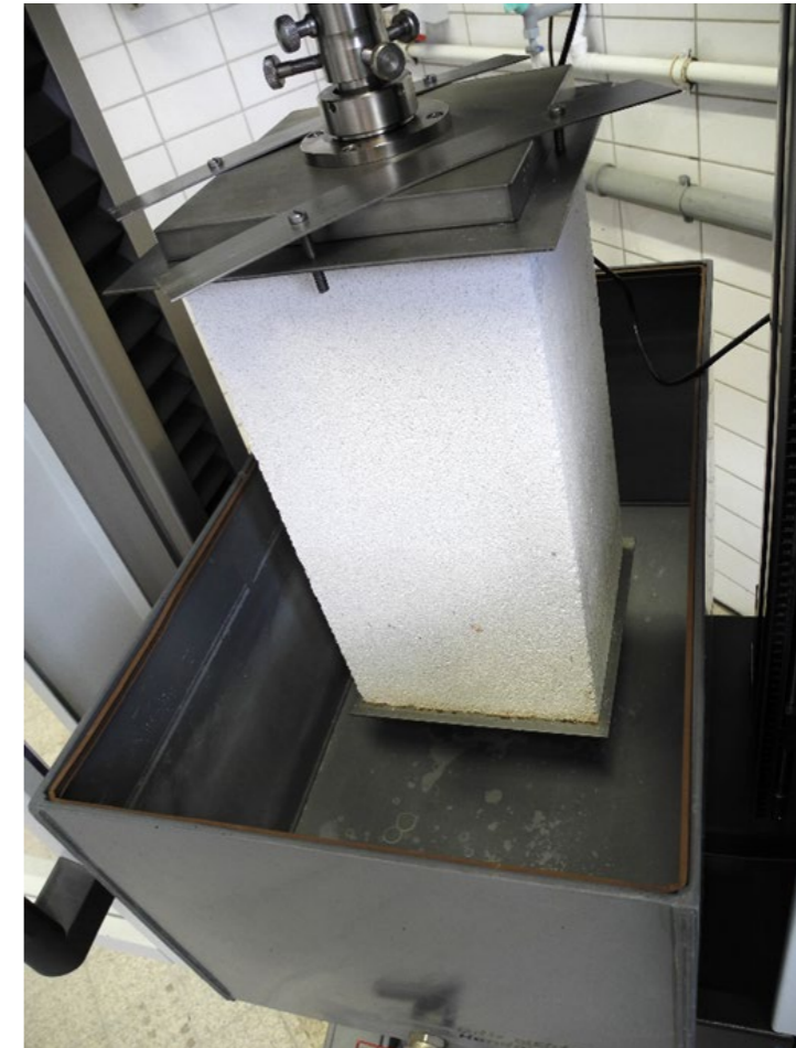
Extension of the testing machine for combined loading: Compression + humidity
