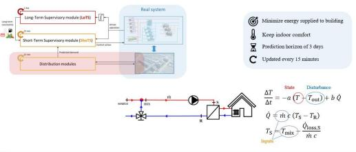
The proposed solution is a multi-level optimal controller with a double timescale which provides the control action every 15 minutes
