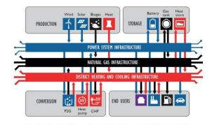
Example of a Hybrid Energy Network with some possible technologies and connections (source: Fraunhofer IEE)
