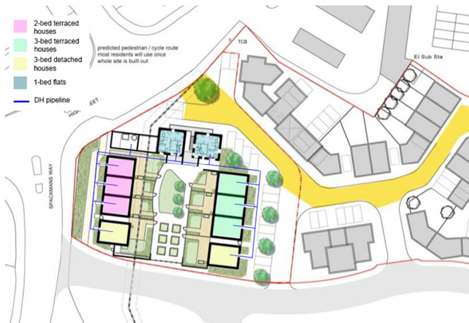
Figure 5. Layout of the district heating network.
