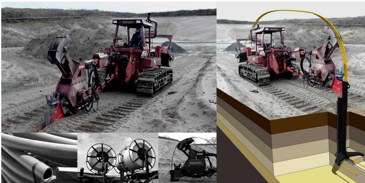
Figure 11. Technology for thermal activation of agricultural fields or other free spaces.
