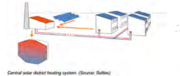
Central solar district heating system. (Source: Solites)
