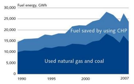
Figure 6.2. Fuel used by conventional and CHP generation.
