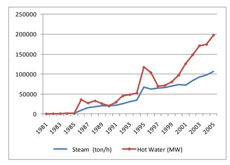
Figure 9.1 Expansion of DH with steam and water as carriers from 1981 till 2007.
