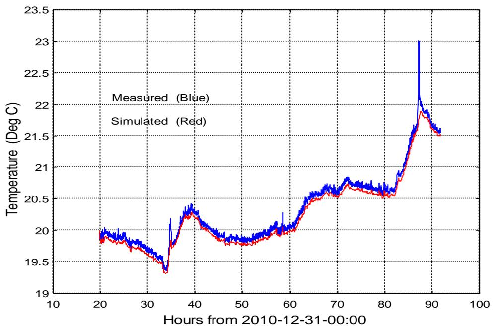
Figure 22: Indoor Temperature during Model Validation Test
