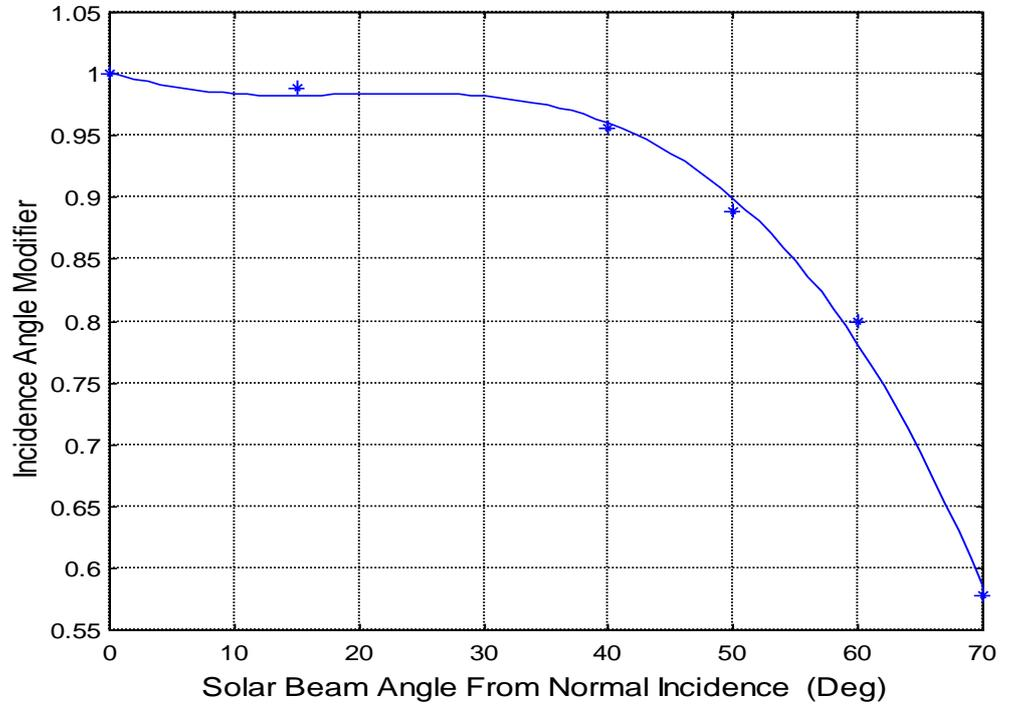
Figure 21: Incidence Angle Modifier for Triple Glazed Window
