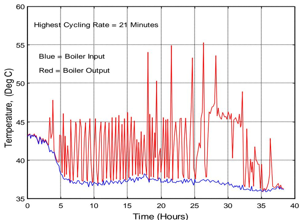
Figure 35: Cycling in a Backup Boiler on a Small DE System
