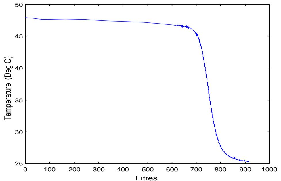
Figure 34: Stratification Performance of Three Tank System at 178 Litres/Hour
