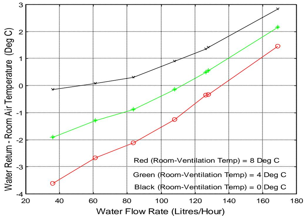
Figure 28: Effect of Ventilation Air Temperature on Water Return Temperature
