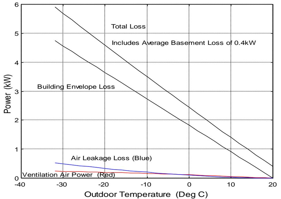
Figure 11: Components of Heat Loss in Dumont House
