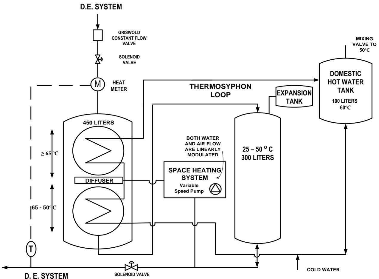
Figure 32: Combined DHW and Building Thermal Storage (Two Tank System)
