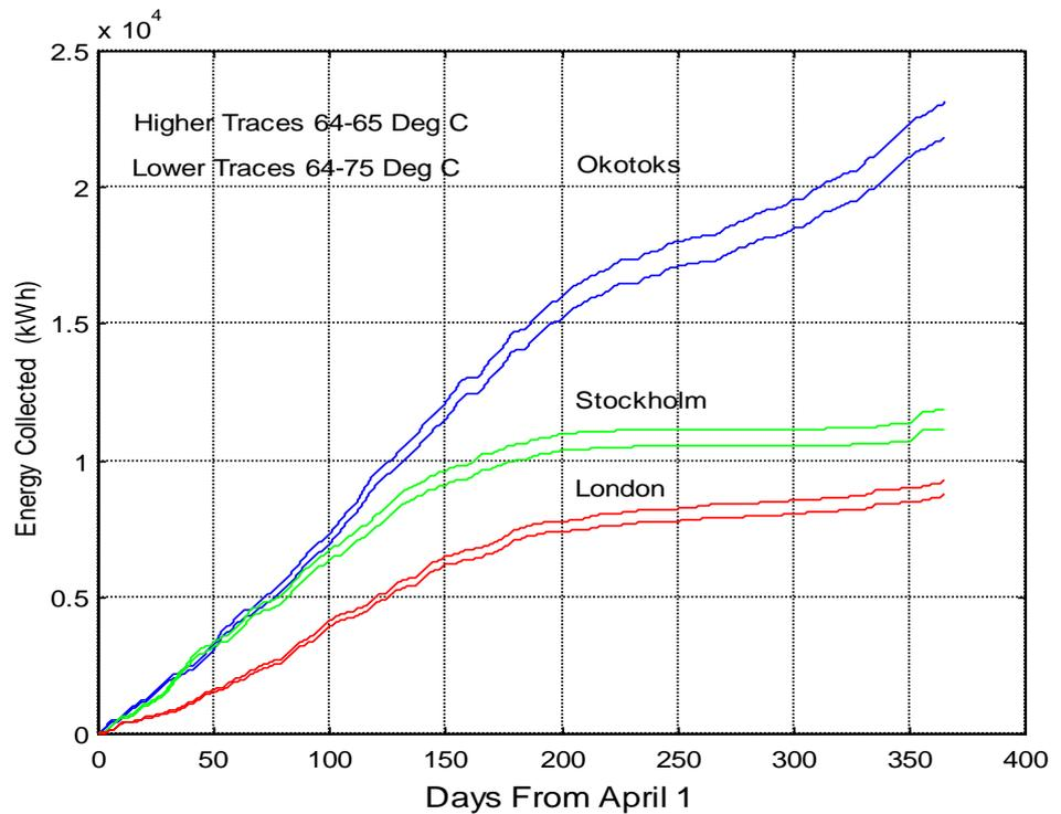
Figure 64: Energy Collected between 64-65 °C and 64-75°C by Collector Array, Tin = 23°C
