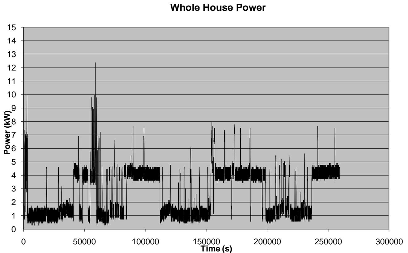
*Figure 9. Whole house electrical power consumption.*
