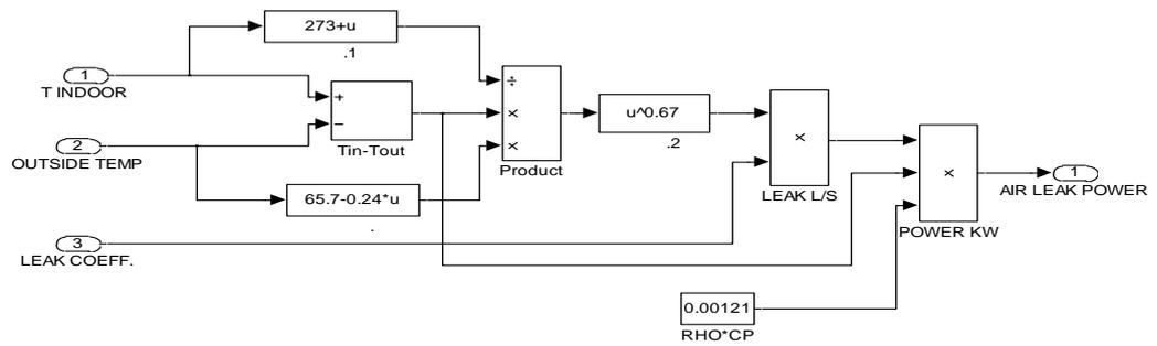
Figure 15: Model for Power Loss due to Air Leakage
