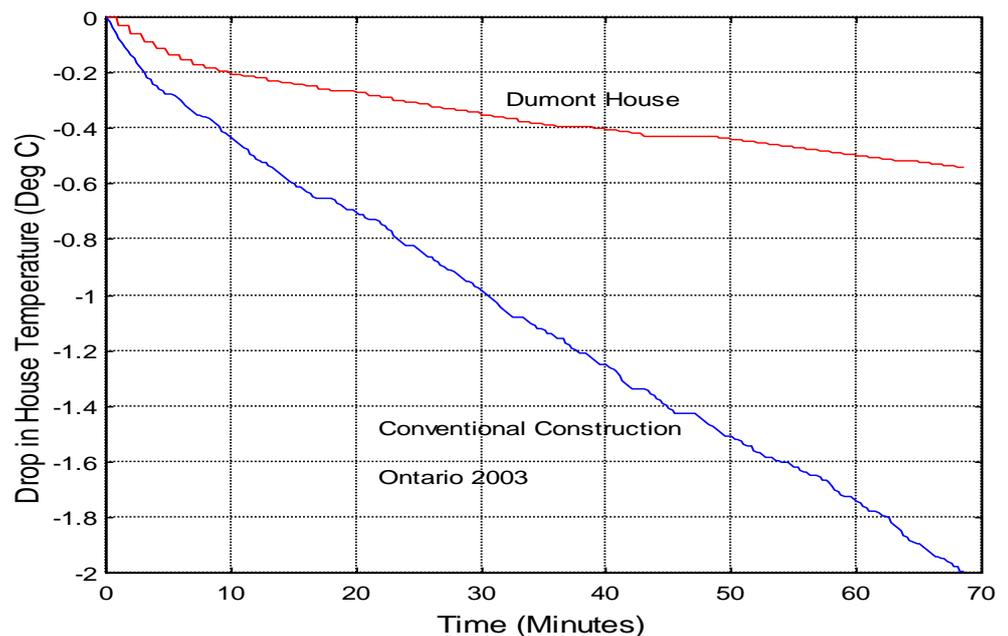
Figure 3: Loss in Temperature with No Space Heat ( $T_{in}-T_{out}$  normalized to  $40^{\circ}\text{C}$ )
