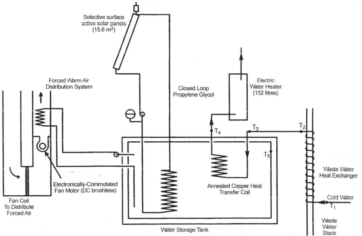
Figure 5. Schematic of the Mechanical Systems in the Dumont Residence
