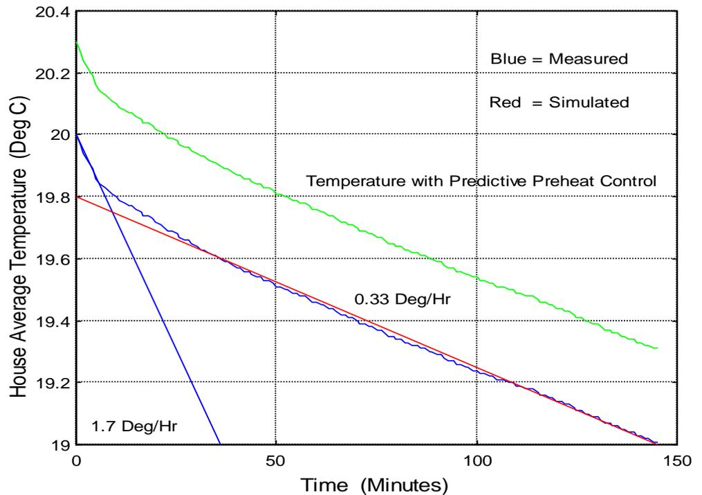
Figure 18: Temperature Changes in Dumont House after Setting the House Space Heating Power to Zero.
