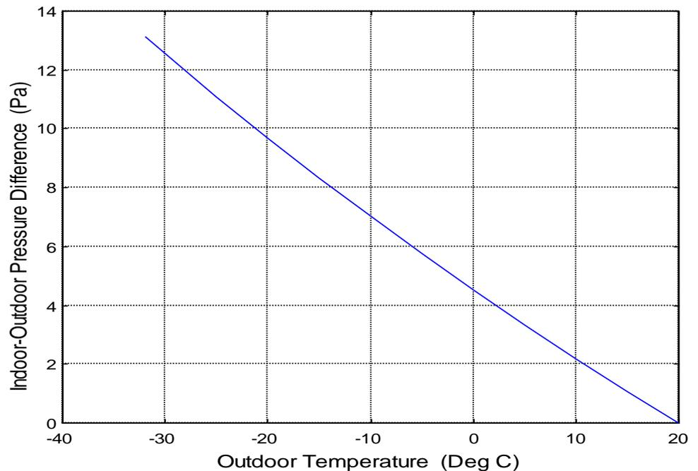
Figure 4: Stack Pressure as a Function of Outdoor Temperature
