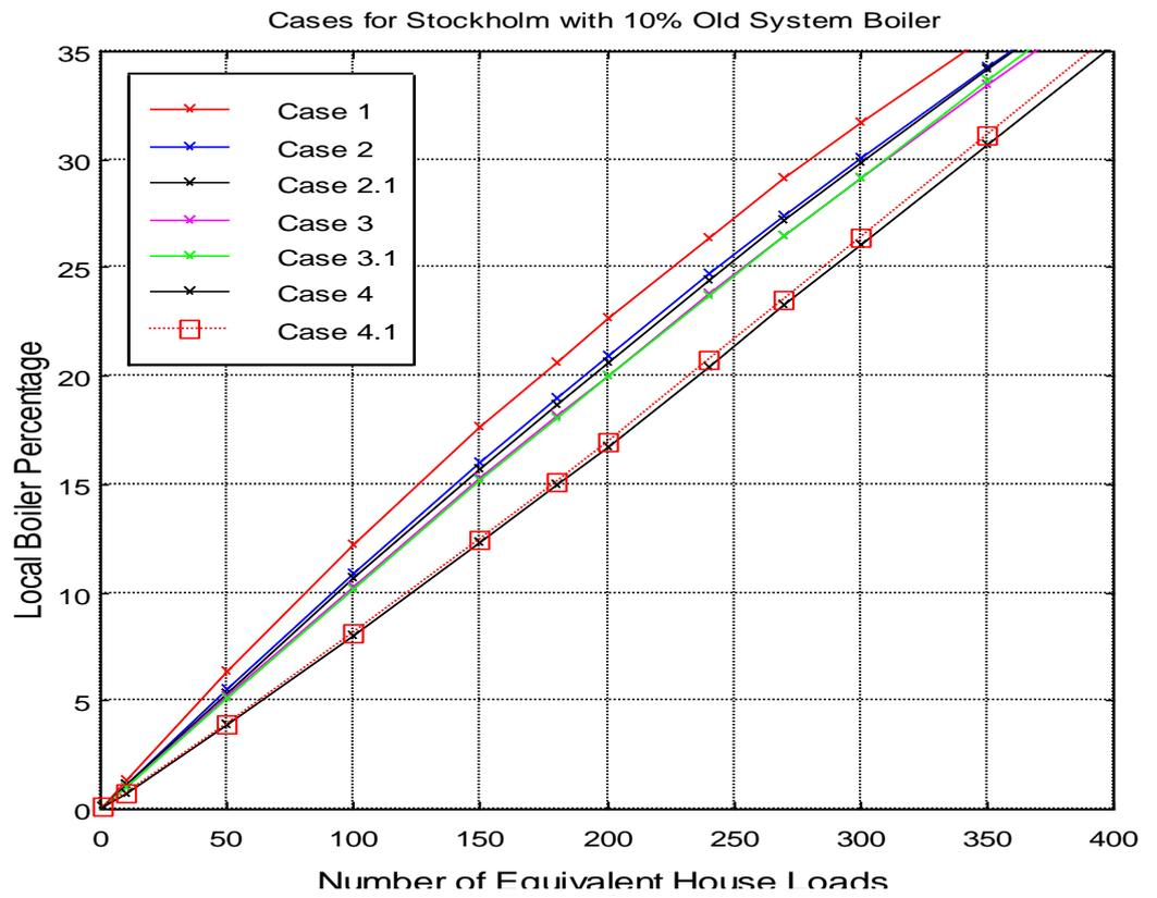
Figure 38: Cases for Stockholm with 10% Old System Boiler
