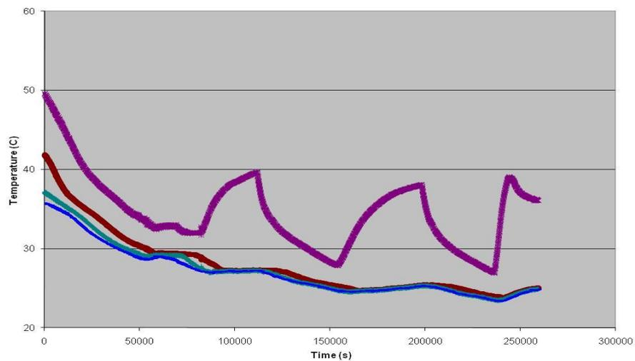
Figure 8: Temperatures in the large storage tank over the three day period with intermittent addition of heat to the tank and heat extraction for space heating.
