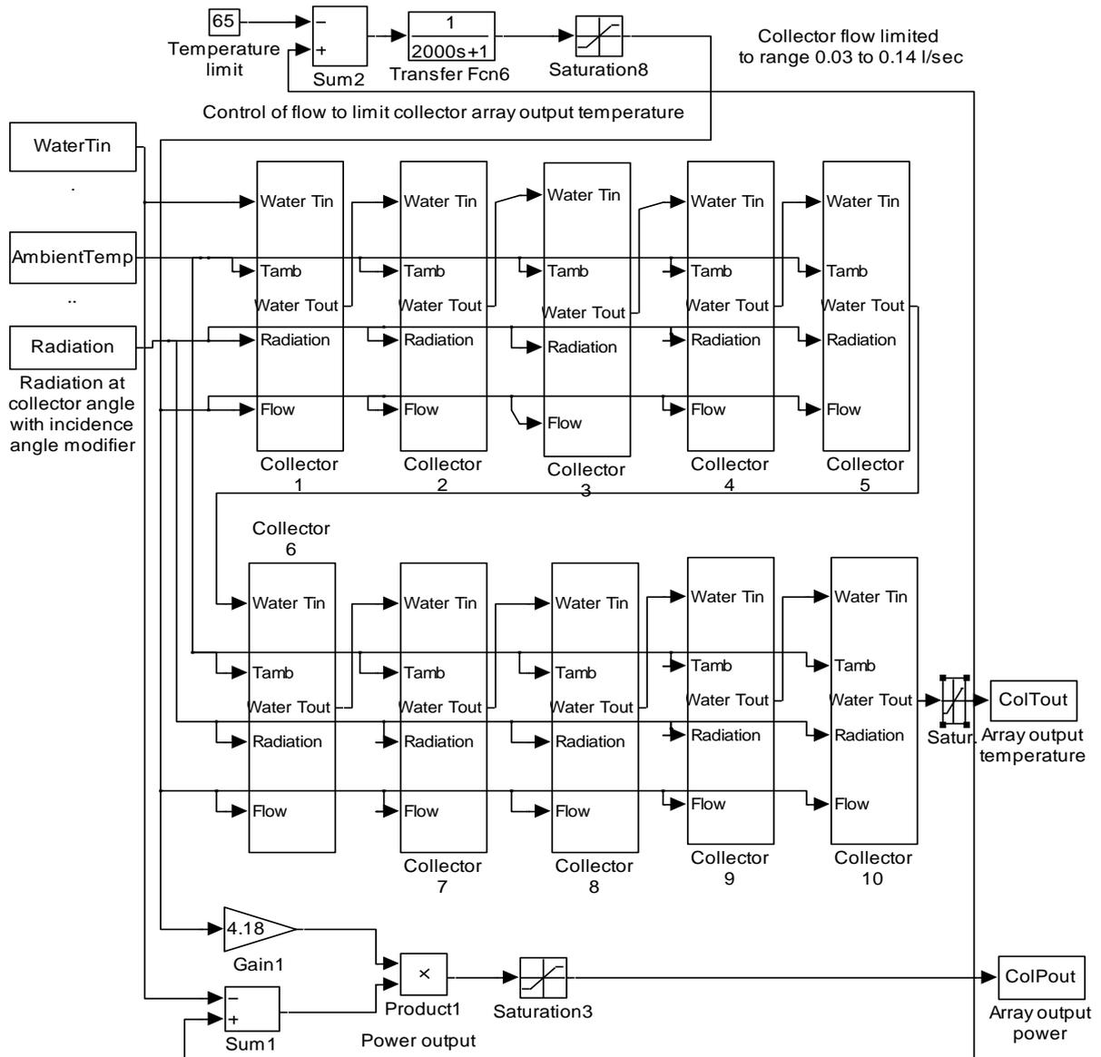
Figure 61: Solar Array with 10 Collectors
