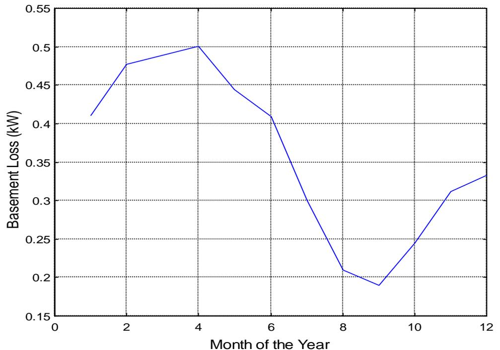
Figure 10: Basement Loss below Grade
