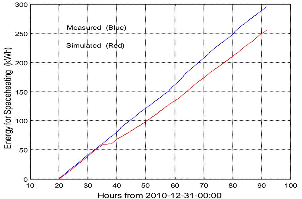
Figure 23: Comparison of Simulated and Measured Space Heat
