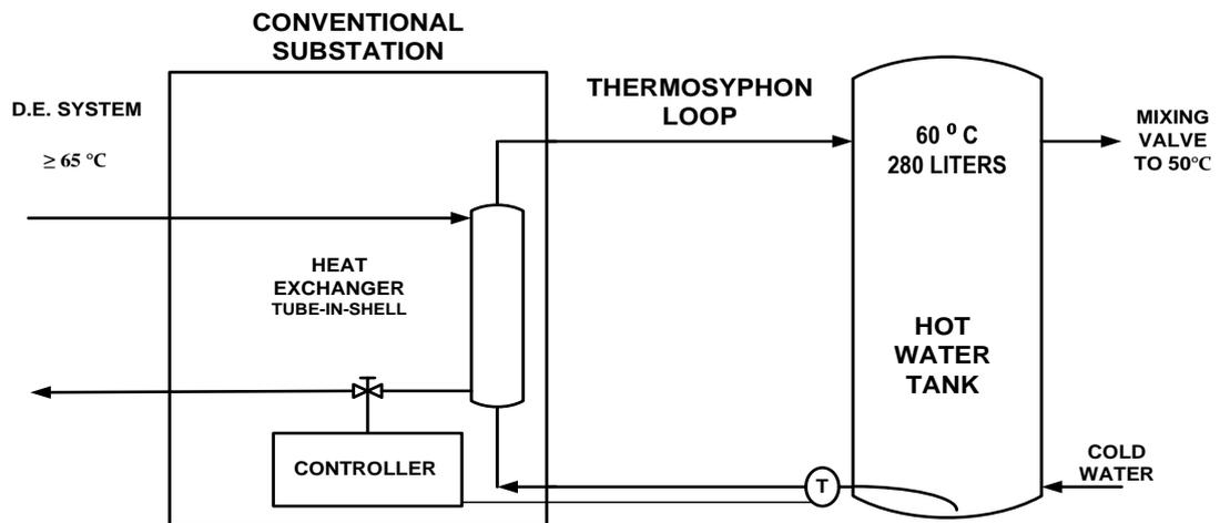
Figure 29: Non-Solar House with Simplified DHW Tank System
