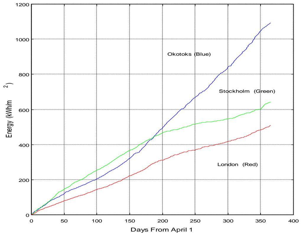
Figure 44: Solar Gain through Window/m<sup>2</sup>
