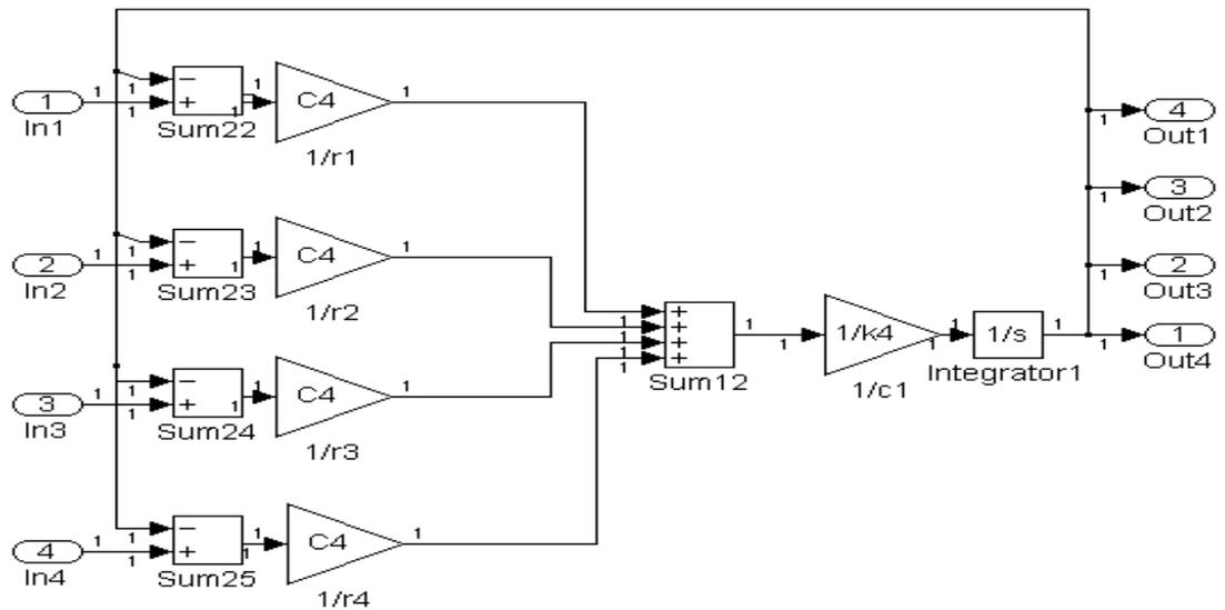
Figure 48: Schematic Representation of One Element of the Borehole Model in SIMULINK™
