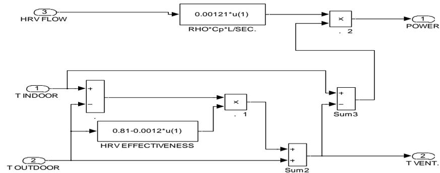
Figure 16: Model for Heat Recovery Ventilator
