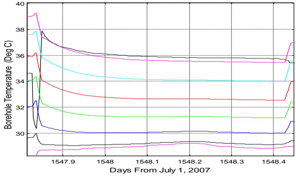
Figure 57: Borehole Simulated and Measured Temperatures at the End of the Discharge Cycle
