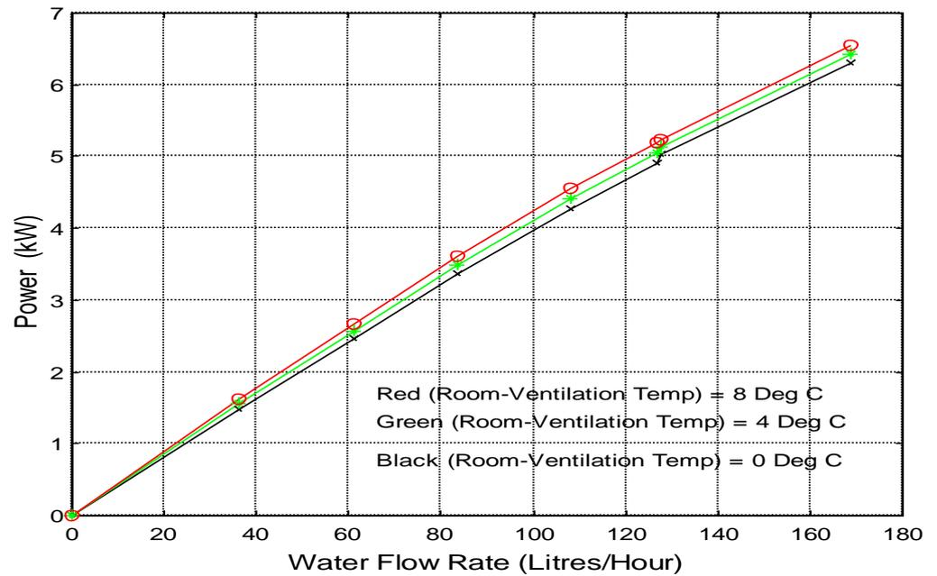
Figure 27: Air Coil Power at Different Ventilation Air Temperatures with Supply Temperature = 65°C
