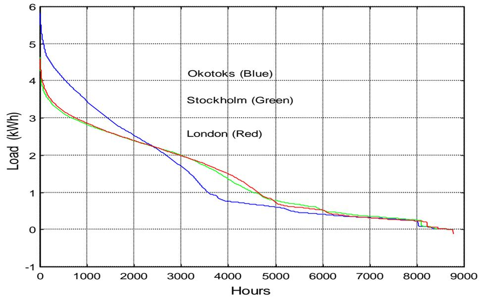
Figure 43: Load Duration Curves for One House
