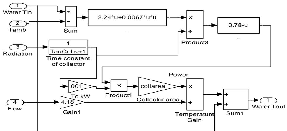
Figure 60: Efficiency and Power Function for a Typical Evacuated-Tube Collector
