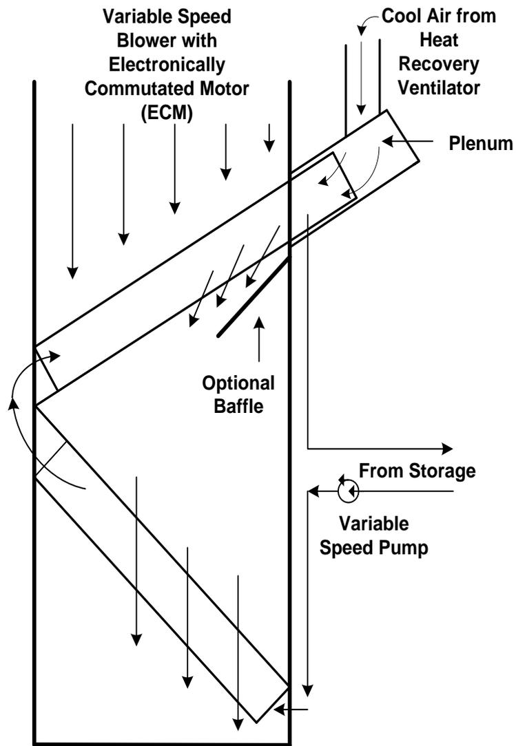
Figure 26: Space Heating System with Single Row Air Coils
