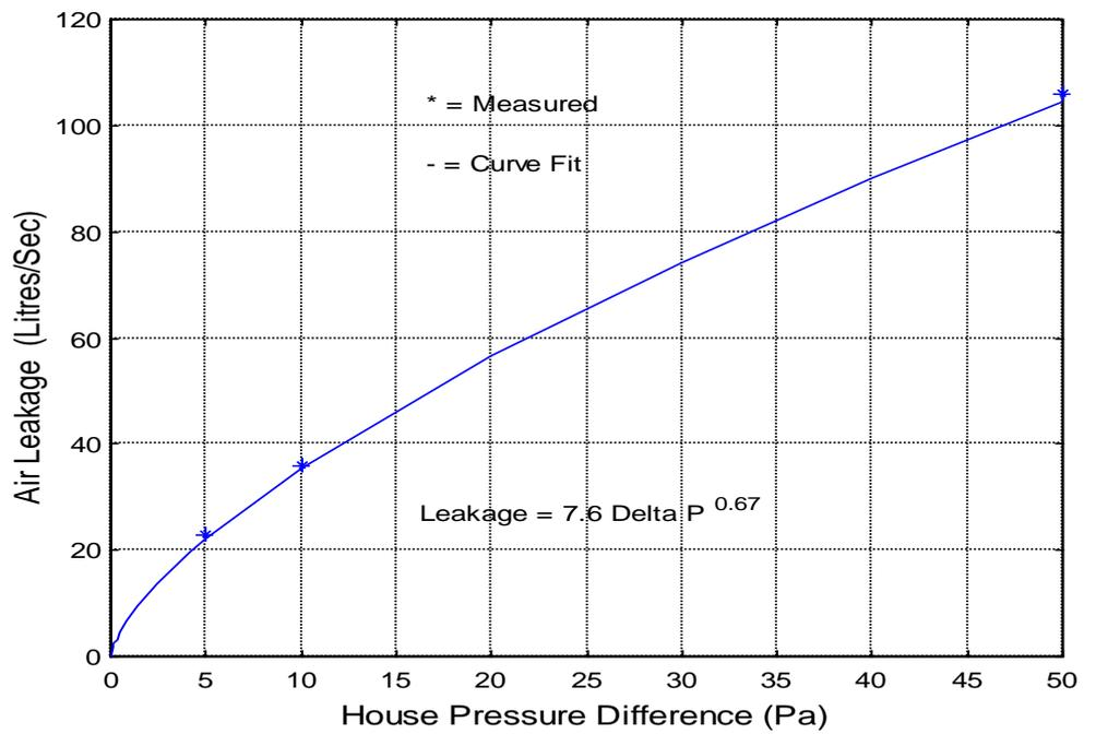
Figure 5: Air Leakage due to Pressurization Test
