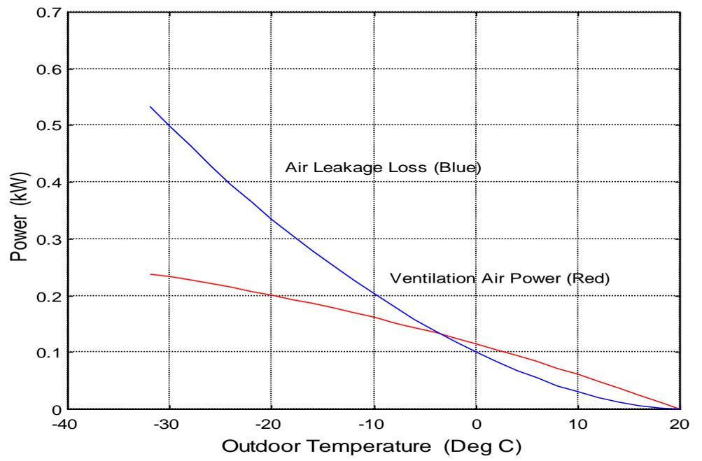
Figure 12: Comparison of Air Leakage Loss and Ventilation Power
