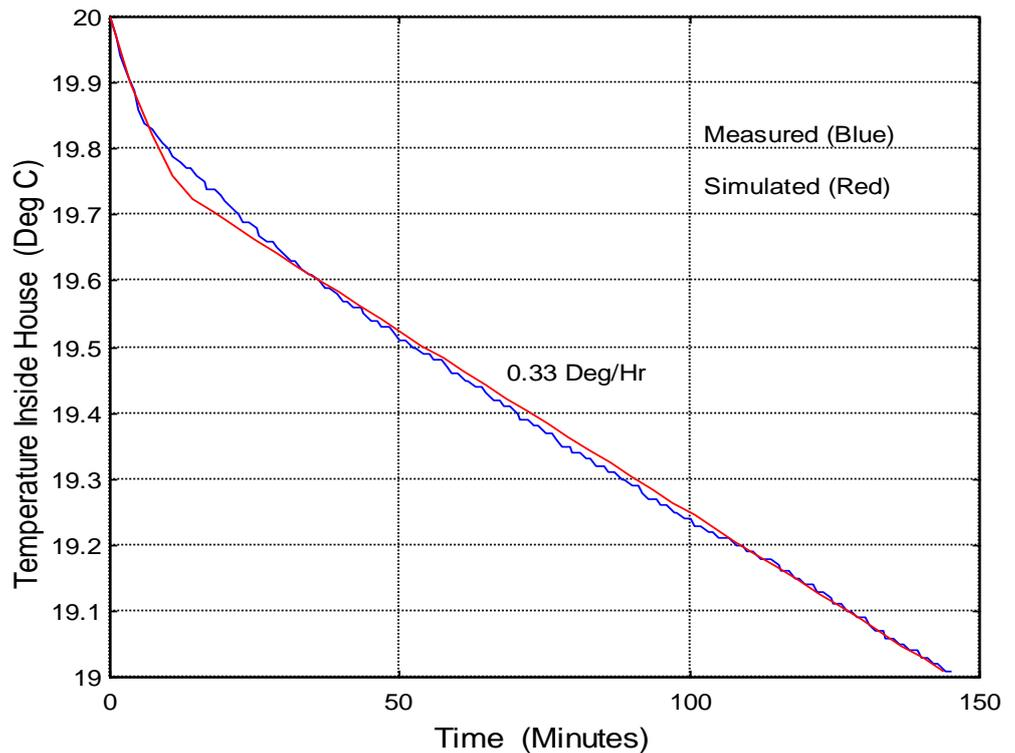
Figure 17: Temperature Drop in Dumont House Normalized to Tin-Tout = 40°C
