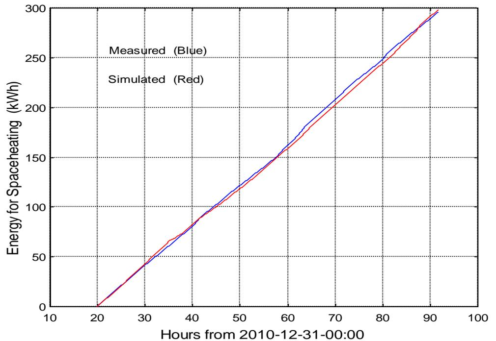
Figure 25: Validation of Dumont House Model with Revised Parameter Set
