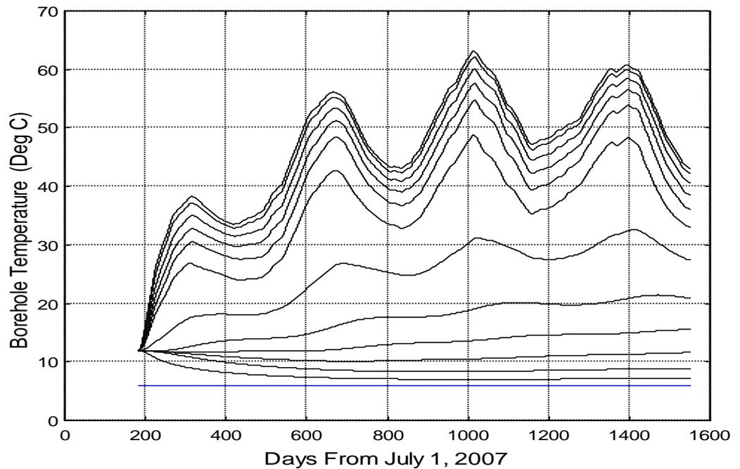
Figure 53: Simulated Temperatures along Line between Boreholes
