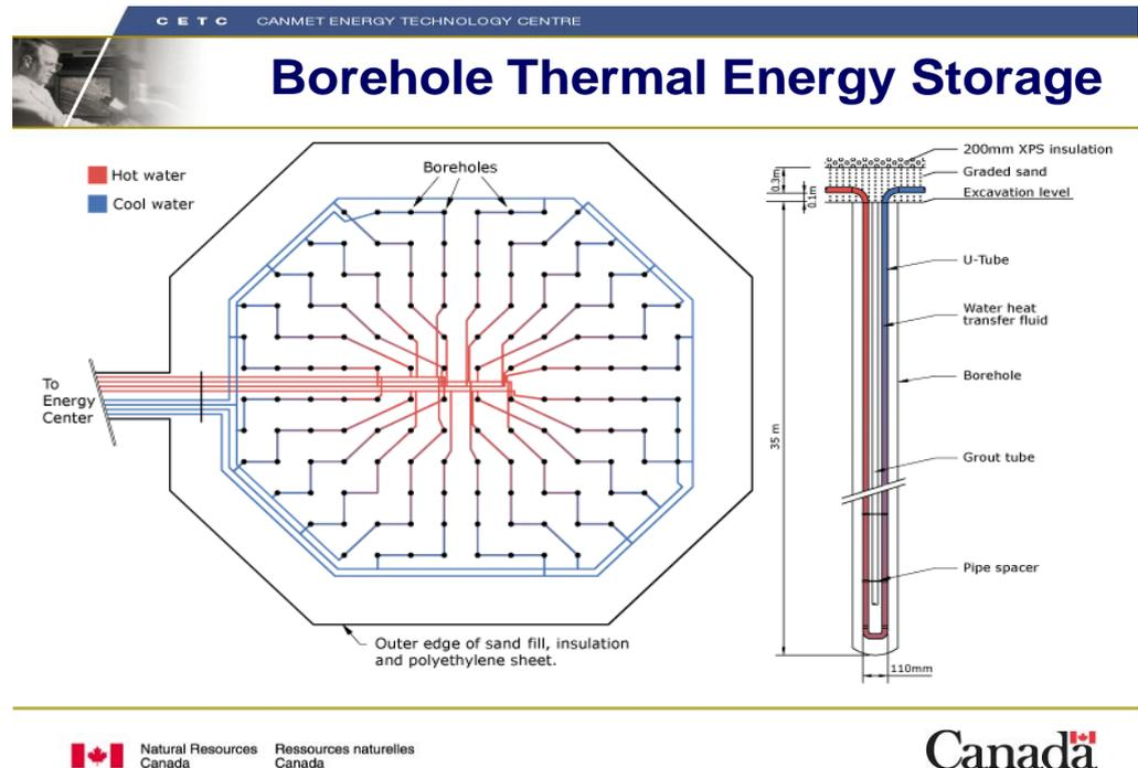
Figure 45: Schematic Diagram of the Okotoks Borehole Thermal Energy Storage
