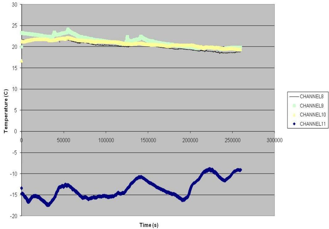
Figure 7. Indoor and Outdoor Temperatures over the three day period
