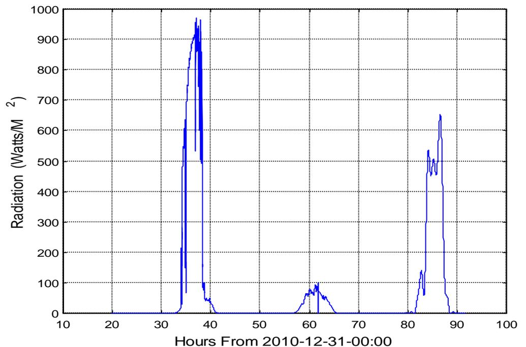
Figure 20: Radiation in Saskatoon on a Vertical South Window
