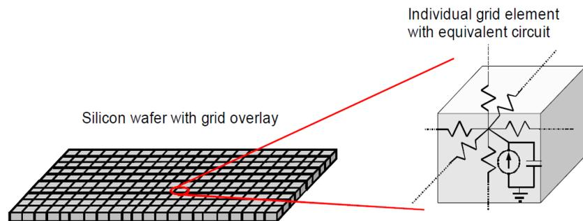
Figure 47: Example of Grid Based Thermal Modeling for Semiconductor Design<sup>35</sup>.
