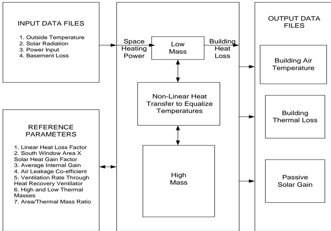
Figure 13: The Block Diagram of the Building Model
