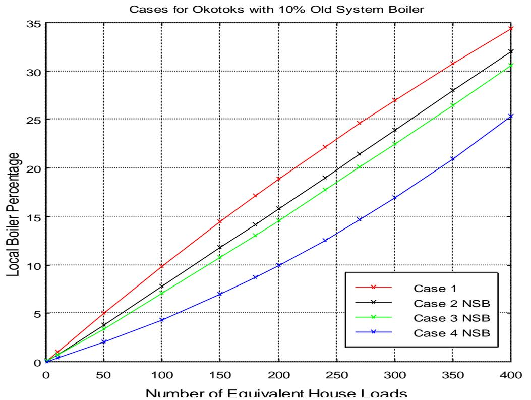
Figure 37: Cases for Okotoks with 10% Old System Boiler using NSB
