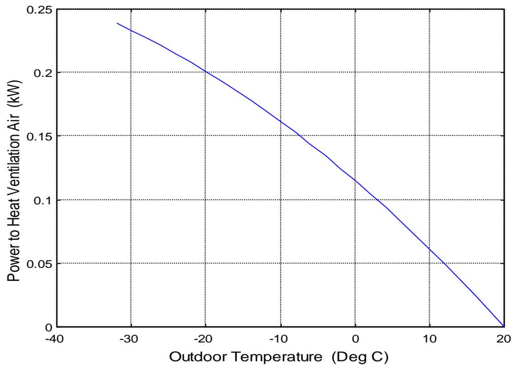
Figure 9: Power to Raise Ventilation Air to 20°C at 25 l/sec
