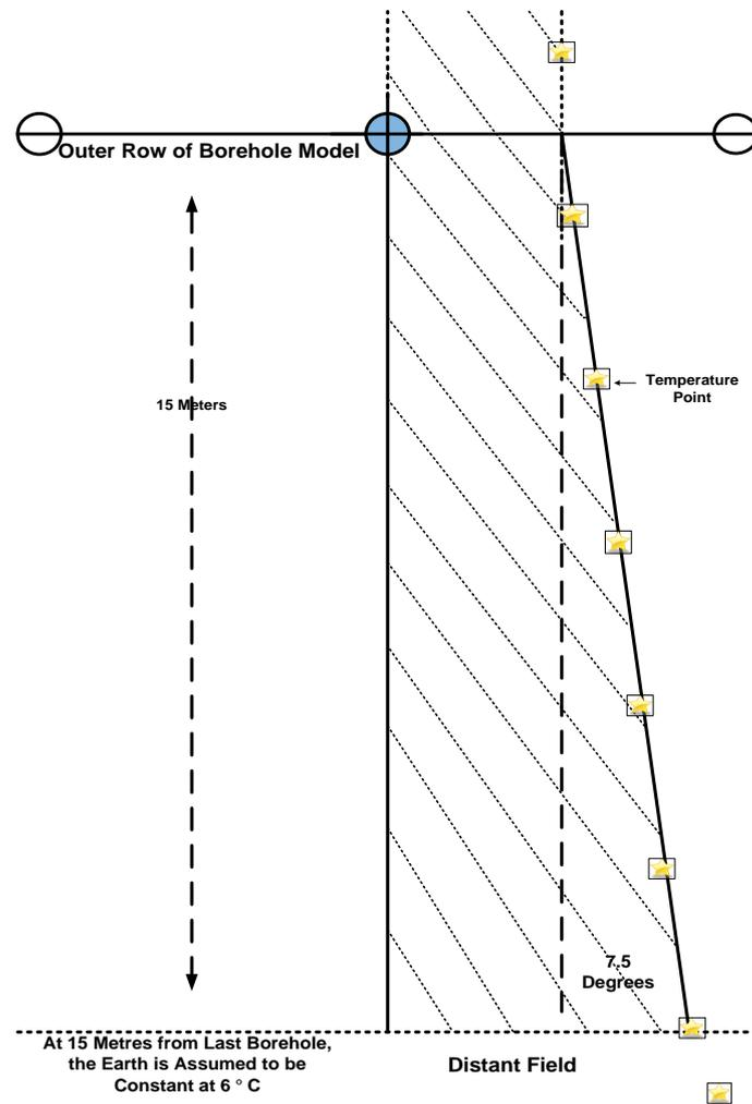
Figure 51: Distant Field outside the Borehole
