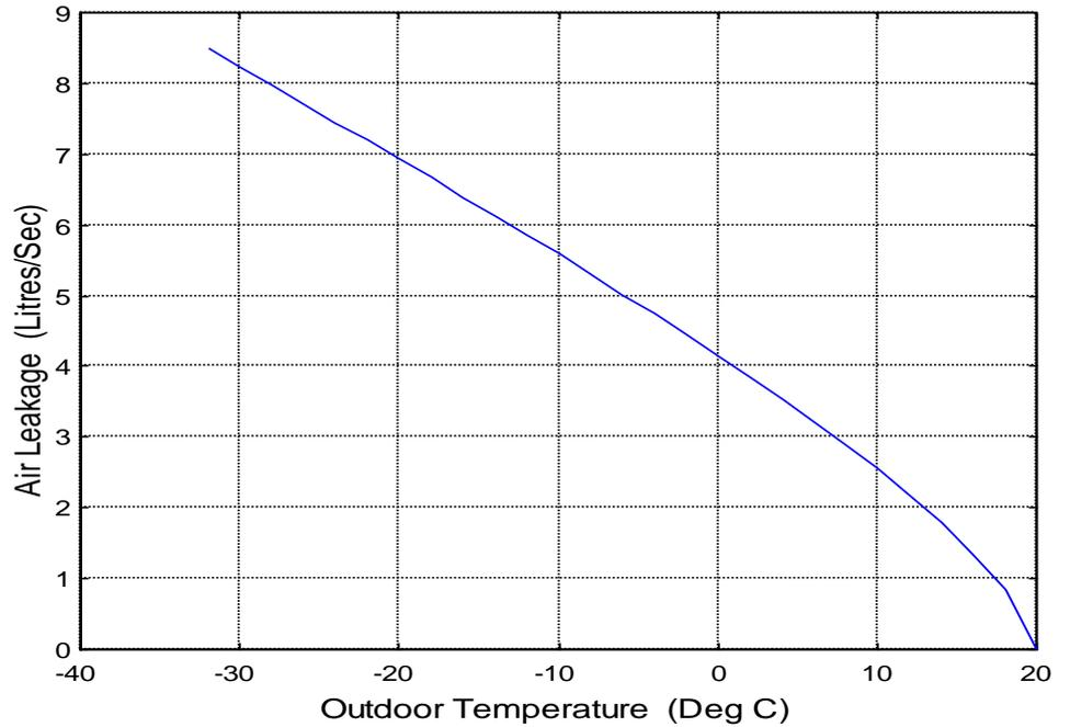
Figure 6: Air Leakage as a Function of Indoor-Outdoor Temperature Difference
