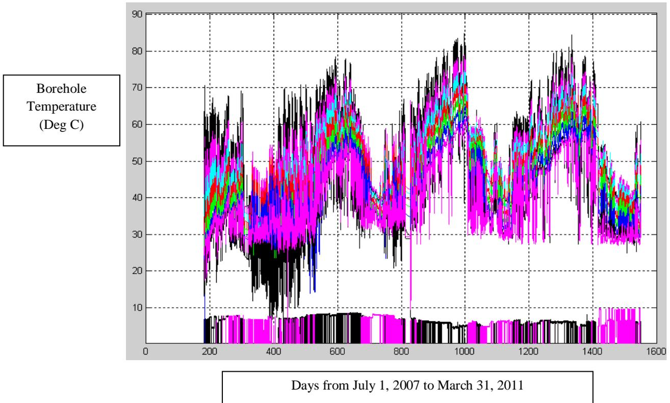
Figure 52: Simulated and Measured Borehole Temperatures at Okotoks<sup>1</sup>
