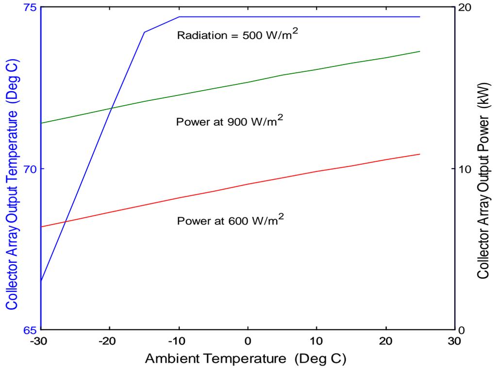
Figure 62: Performance of 10 Collector Array with Okotoks Weather,  $T_{in} = 30^{\circ}\text{C}$
