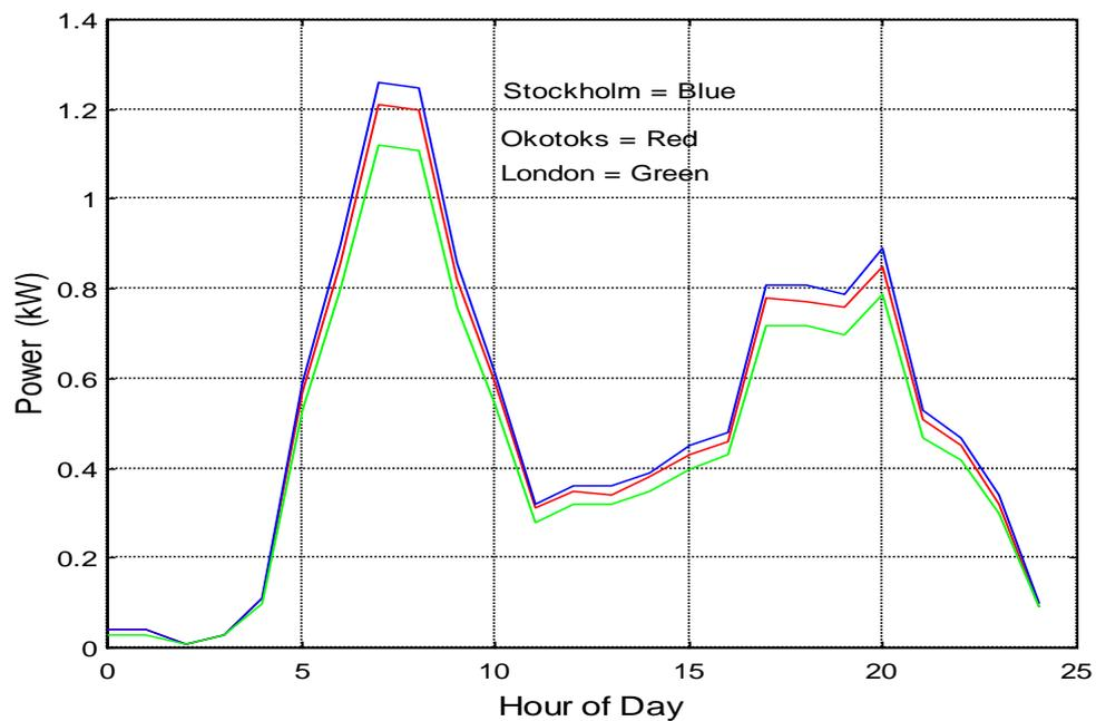
Figure 31: DHW Power per House, Diversified for 240 Houses
