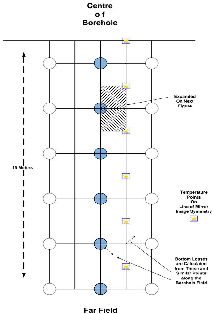
Figure 49: Schematic Drawing of Borehole and Far Field
