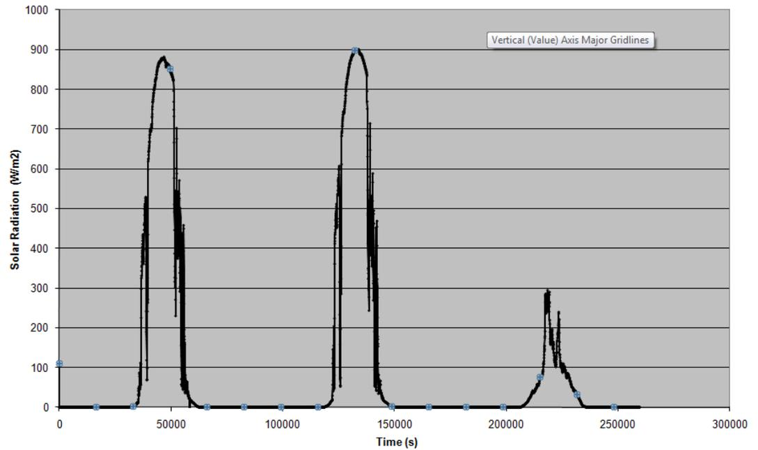
*Figure 6. South Vertical Incident Solar Radiation from December 20 to 23, 2010*
