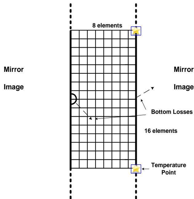
Figure 50: Expanded Schematic of Borehole Grid
