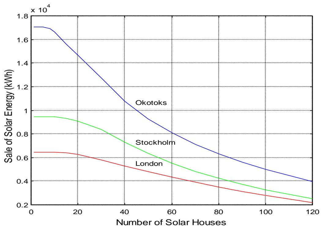
Figure 65: Solar Energy Transferred Directly to Non-Solar Houses
