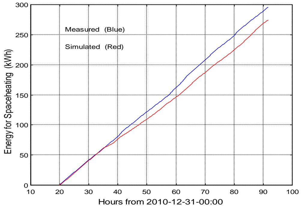
Figure 24: Comparison of Simulated and Measured Space Heat
