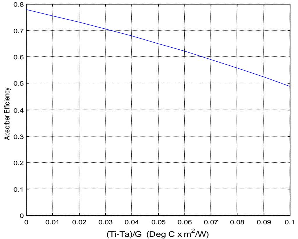
Figure 59: Typical Absorber Efficiency of an Evacuated Tube Collector
