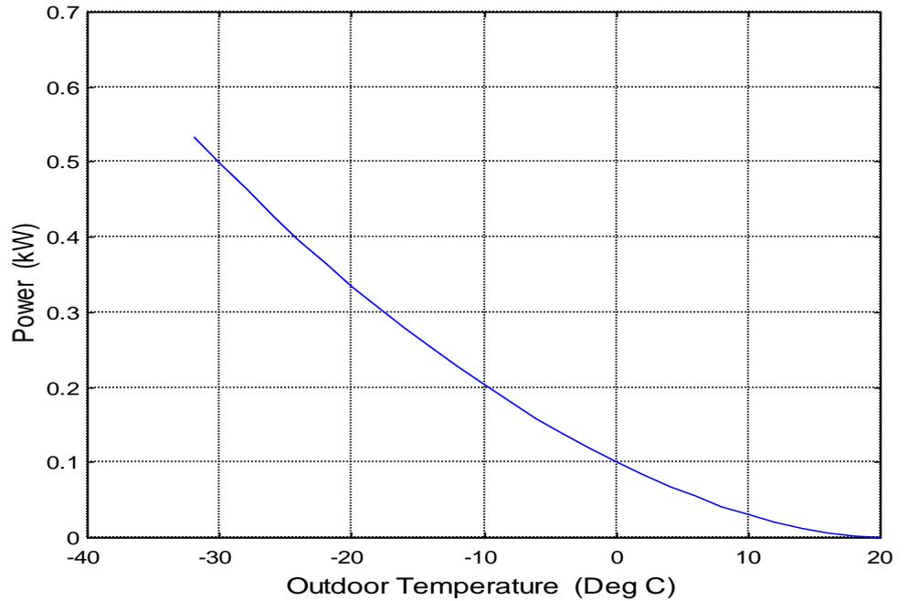
Figure 7: Power Required to Heat Air due to Leakage
