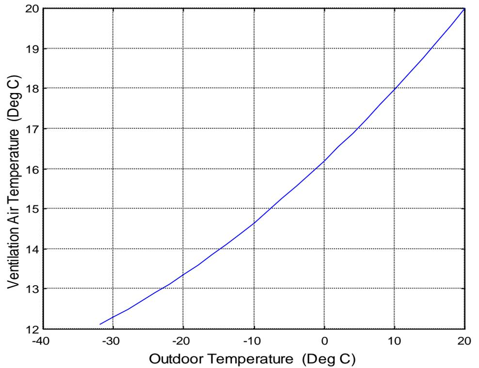
Figure 8: Ventilation Air Temperature from HRV
