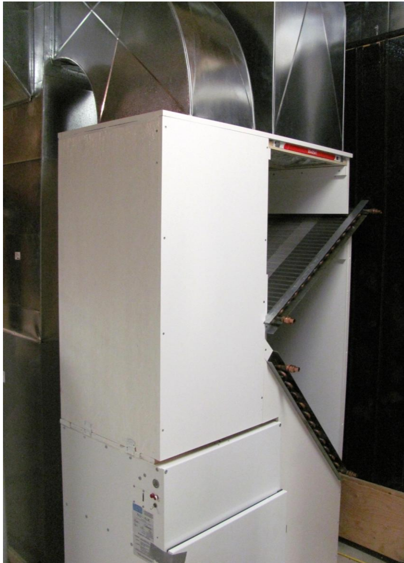
Figure 11: Space Heating System Prototype with Single Row Air Coils
