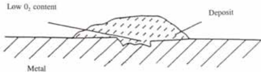
Fig. 4.1.4 Example of deposit corrosion. Concentration differences in oxygen contents provide sufficient force to make the metal under the deposit form an anodic surface and corrode. The higher O_2 content in the electrolyte functions as a cathodic surface.
