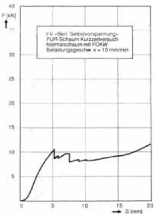
Figure 8-1: Force/displacement
