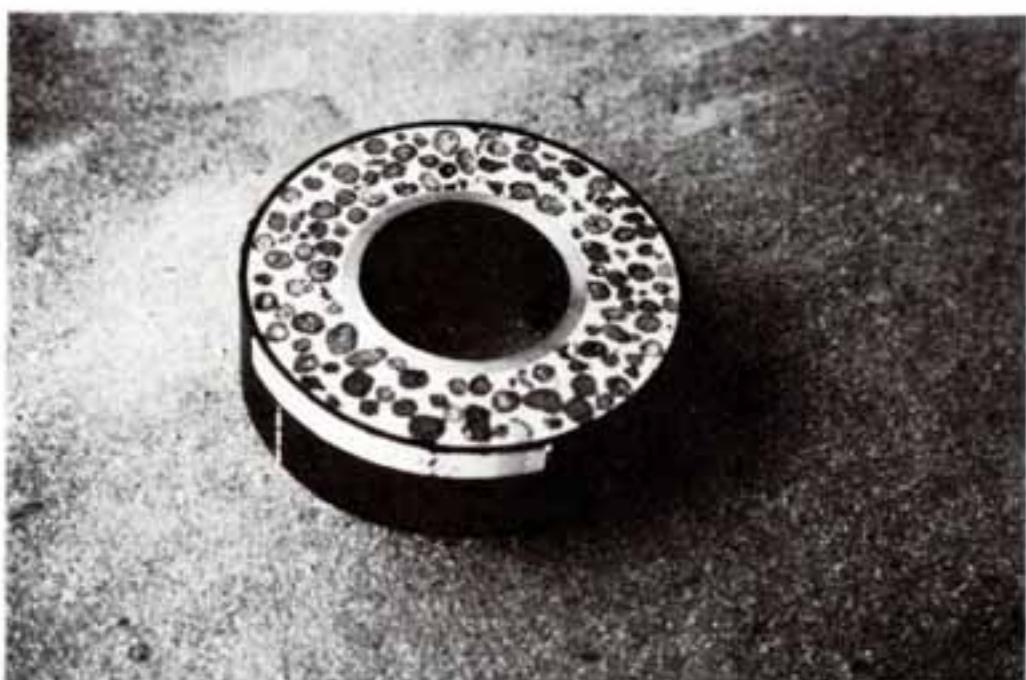
Figure 6-2: Actual type of pipe able to withstand high transverse loadings.
