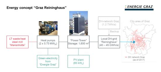
Figure 81. Supply of the new urban district "Graz Reininghaus" with an innovative heat supply concept. Adapted from (Unger, 2018).
