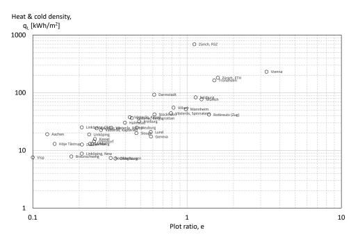
Figure 68. Combined heat and cold density as a function of the plot ratio.
