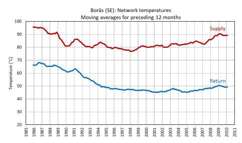
Figure 37. Supply and return temperature in the Borås (SE) district heating network. Source: (Dahlberg & Werner, 1997) complemented with later years.
