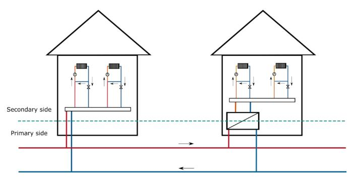
Figure 50. Directly and indirectly connected substations of the current system at TU Darmstadt Campus Lichtwiese.
