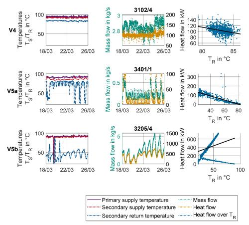
Figure 60. Temperatures, mass flow, heat flow, and heat flow over TR for the two categories V4 & V5 of faulty ventilation heating circuits, including a distinction between categories V5a and V5b.
