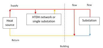
Figure 93. General layout for the supply-to-supply variant of the Warm – Classic configuration
