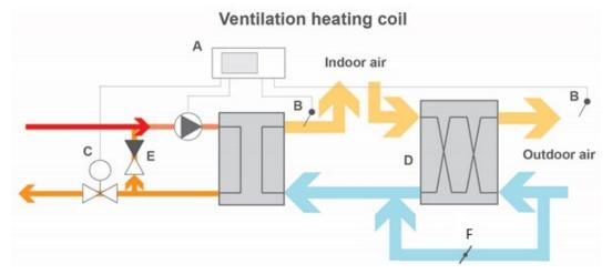
Figure 24. Example of the layout of a ventilation heating coil in a ventilation system where heat recovery is bypassed due to cold outdoor temperature. (A) Controller, (B) Temperature sensor, (C) Control valve, (D) Heat recovery unit, (E) District heating bypass and (F) Bypass damper.
