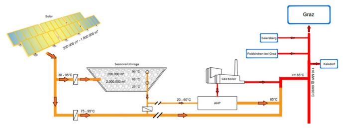
Figure 43. Scheme of the BIG Solar Graz concept (Reiter et al., 2016)
