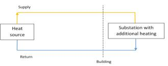
Figure 97. General layout for the Cold – Ultra-Low configuration
