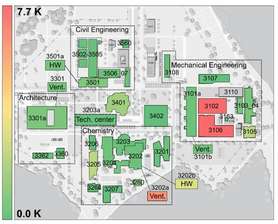
Figure 53. Return temperature reduction potential for each substation at Campus Lichtwiese.
