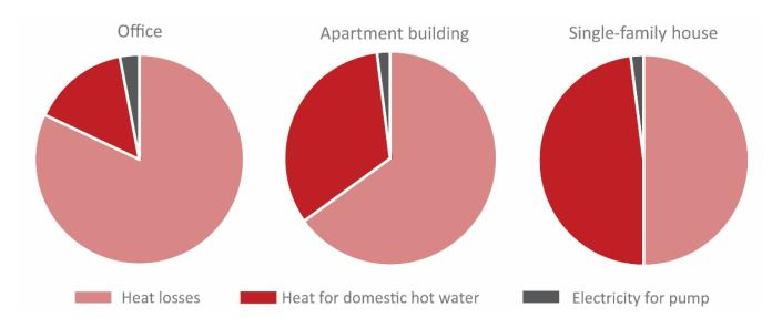
Figure 21. Energy use for typical Danish domestic hot water installations (based on Bøhm, Schrøder, et al., 2009)
