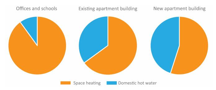
Figure 20. Shares of heat for domestic hot water and space heating in three different building types in Denmark (based on Bøhm, Schrøder, et al., 2009)
