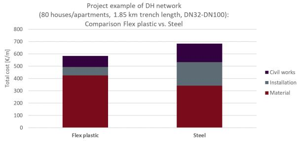
Figure 17. Total costs of a completed example project installed in a smaller district heating network (Engel, 2020)
