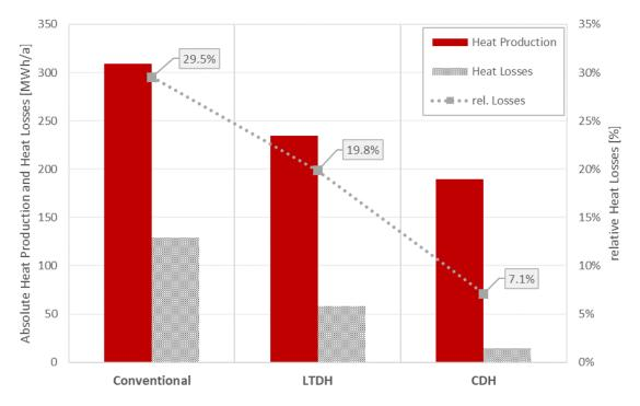
Figure 48. Comparison of different supply concepts and their network losses for a mixed-use neighbourhood in Amstetten (AT) with access to conventional high-temperature district heating (Leppin, 2020)
