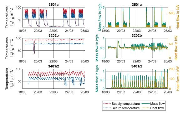
Figure 56. Temperatures, mass flow, and heat flow of the heat circuits supplying hot water.
