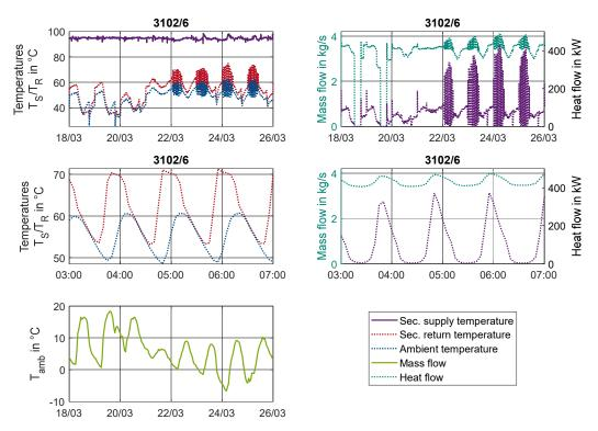
Figure 58. Temperatures, mass flow, and heat load of the faulty space heating circuit 3102/6.
