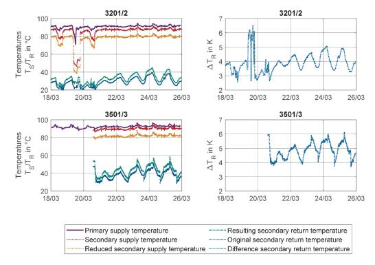
Figure 61. Temperatures before and after supply temperature reduction for the heating circuits 3201/2 and 3501/3
