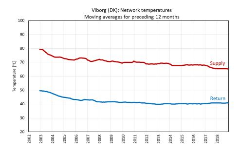
Figure 36. Supply and return temperature in the Viborg (DK) district heating network (Diget, 2019)
