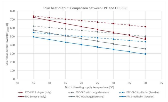
Figure 11. Comparison of specific solar heat output for flat plate collectors (FPCs) and evacuated tube collectors with compound parabolic concentrator (ETC-CPCs) at various district heating supply temperatures (direct feed-in unit, return-to-supply feed-in, with pre-heating loop, without storage) for five different locations
