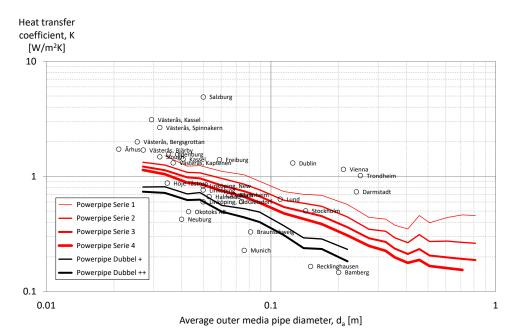
Figure 73. Annual average heat transfer coefficient as a function of the average pipe diameter.
