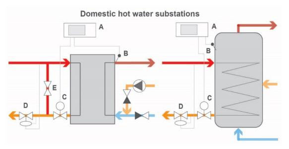
Figure 23. Example of the layout of a domestic hot water heat exchanger (left) and a domestic hot water storage tank (right). (A) Controller, (B) Temperature sensor, (C) Actuator and control valve, (D) Differential pressure controller, and (E) Bypass valve (may be located internally in the unit).
