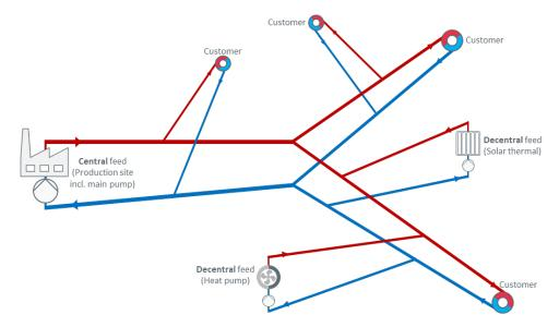
Figure 44. Ilustrative pressure levels for a district heating network with centralised and decentralised heat sources.
