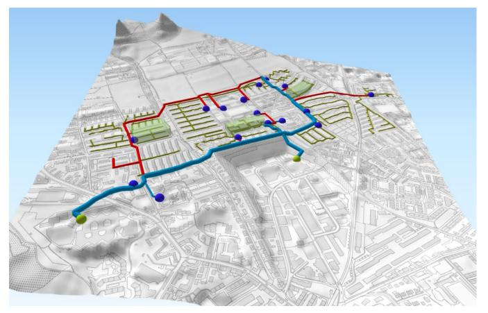
Figure 79. Layout of the FGZ cold district heating system including heat sources, borehole storages, heat pump locations and secondary distribution network sources: AEE INTEC, anex Ingenieure AG, opendata.swiss
