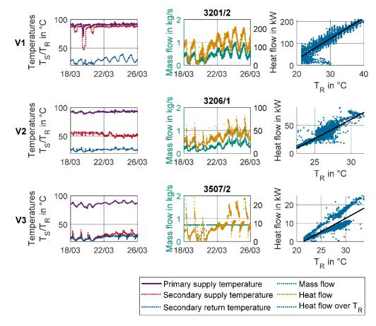
Figure 59. Temperatures, mass flow, heat flow, and heat flow over return temperature for the categories V1-V3 of well-functioning ventilation heating circuits.
