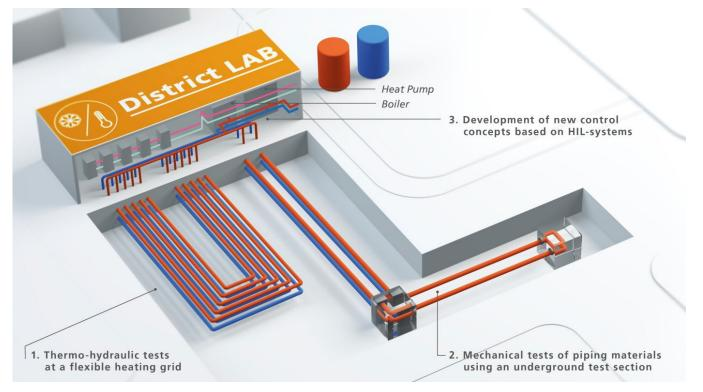
Figure 90. The system layout from the District LAB test facility for innovative district heating systems on a community scale, © Fraunhofer IEE
