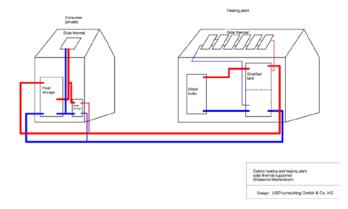
Figure 77. Integration of the solar thermal system into the grid (Source: UBP-consulting GmbH & Co.KG)
