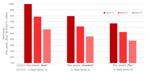
Figure 46. Comparison of heat loss values for flexible plastic pipes of different insulation classes at different temperature levels (Basic at 95/65 °C = 100%) (Austroflex Rohr-Isoliersysteme GmbH, 2020)
