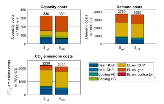
Figure 65. Impact of the proposed temperature reduction measures on the capacity-related, demand-related, and carbon dioxide emission costs.
