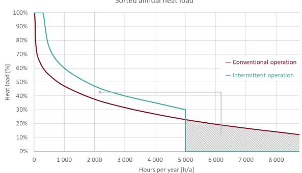
Figure 49. Qualitative visualisation of sorted annual heat load curves for conventional and intermittent operations (modified from Hammer et al., 2018)
