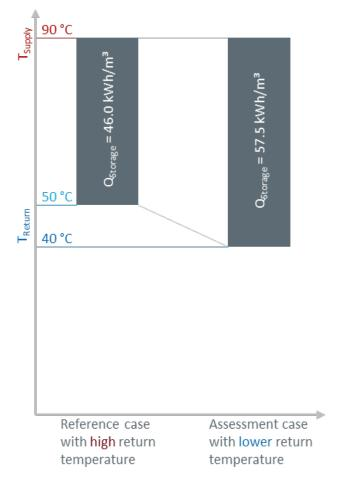
Figure 15. Impact of temperature spread on storage capacity
