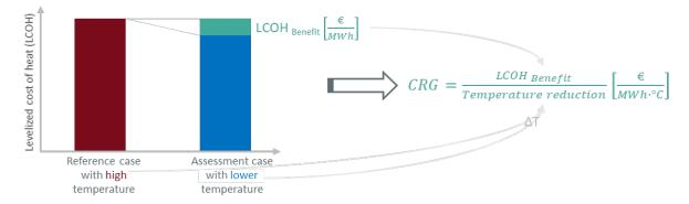
Figure 8. Concept of the energy-economic assessments with the key performance indicator 'cost reduction gradient' (CRG) in euro/(MWh·°C) (Gever, 2020)
