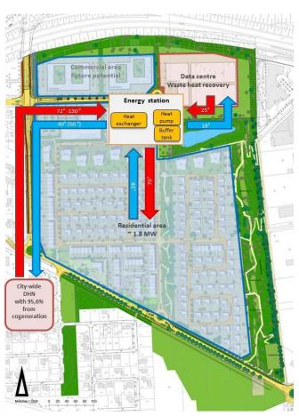
Figure 82. Excess heat recovery from data centre in Braunschweig/Germany.
