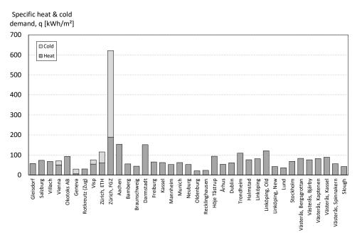
Heat and cold densities assess the concentration of heat and cold deliveries (output at substations) on a given land area. This output parameter assesses the to-
