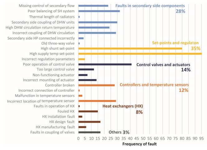
Figure 26. Categorization of 520 faults identified in 246 Swedish substations with high return temperatures. The figure is based on Figure 10.21 in Frederiksen & Werner, 2013, which has been updated based on personal communication.
