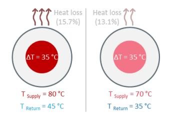
Figure 16. Example of heat loss in a district heating network for design system temperatures (80/45 °C, left) and reduced system temperatures (70/35 °C, right)
