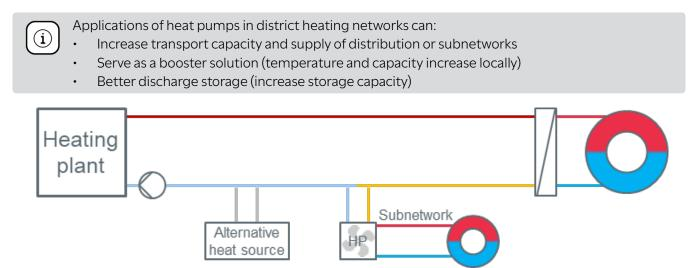
Figure 42. Integration of heat pumps with internal heat sources. On the one hand, this reduces the return flow; on the other hand, this increases capacity (modified from Geyer et al., 2019)
