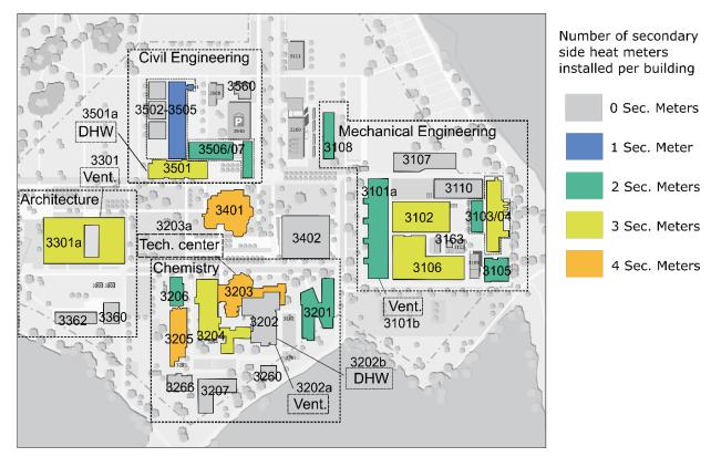
Figure 52. Primary and secondary side heat meters at Campus Lichtwiese.
