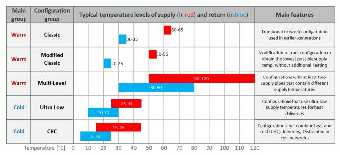
Figure 47. Overview of the network configurations and classifications this guidebook provides for low-temperature heat distribution, including typical temperature levels and principal features
