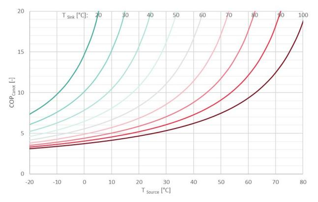
Figure 10. Characteristics of achievable COP<sub>Carnot</sub> as a function of sink and source temperatures
