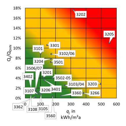
Figure 55. Heat demand  $Q_i$  of each substation j in relation to total heat demand  $Q_{_{DHN}}$  vs. area-specific heat demand  $q_j$
