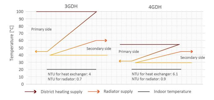
Figure 28. Example showing the difference between the design of a heat exchanger for space heating in an old district heating system and the design of a heat exchanger intended for 4GDH.
