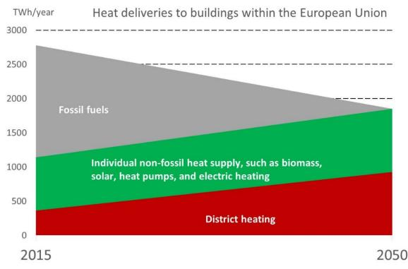
Figure 1. Possible transition from the current heat supply (expressed with the origins of the supply) to buildings within the EU being fully decarbonised by 2050, according to the Heat Roadmap Europe cluster project.
