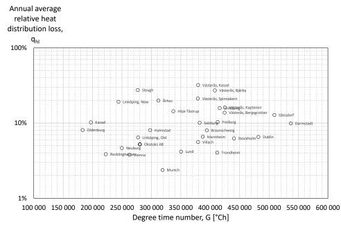
Figure 71. Relative annual heat distribution loss as a function of the temperature level expressed with the annual degree time number.
