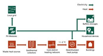
Figure 86. Scheme of the energy system concept in Lagarde Campus Bamberg / Germany © Fraunhofer IEE
