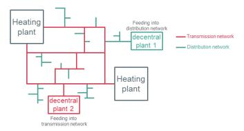
Figure 40. Feed-in points of distributed generators in a meshed heat network featuring transmission and distribution sections
