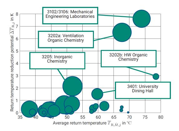
Figure 54. Return temperature reduction potential over average return temperature for each substation at Campus Lichtwiese.
