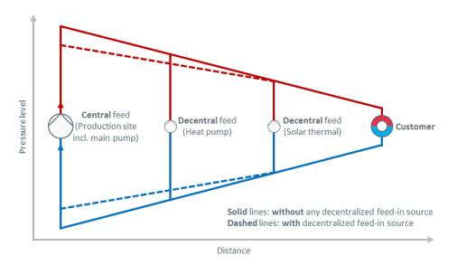
Figure 45. Visualisation of a district heating network showing centralised and decentralised heat sources and flow directions (modified from Nagler & Ponweiser, 2018)
