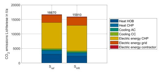
Figure 64. Impact of the proposed temperature reduction measures on CO<sup>2</sup> emissions.
