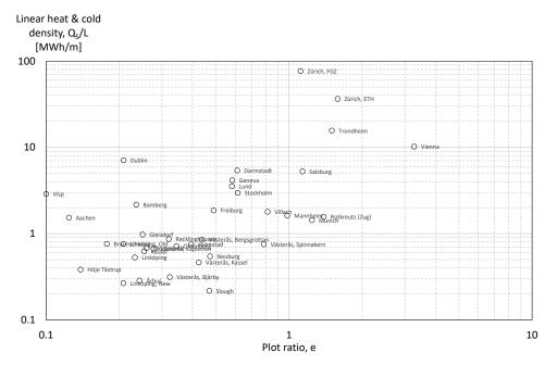
Figure 69. Combined linear heat and cold density as a function of the plot ratio.
