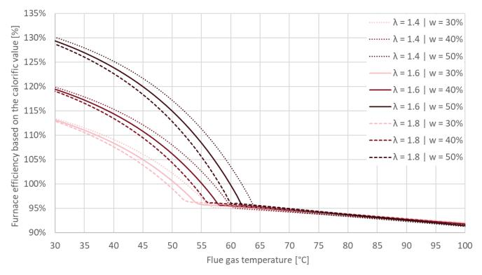
Figure 12. Furnace efficiency of a biomass boiler (according to lower calorific value) as a function of flue gas temperature using wood chips as fuel (w = water content;  $\lambda$  = excess air number).
