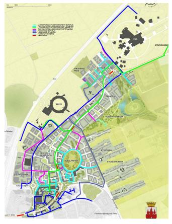
Figure 83. The planned Brunnshög low-temperature heat distribution network. © Kraftringen Energi AB.
