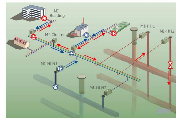
Figure 78. Scheme of Mijnwater combined heating and cooling configuration cluster concept
