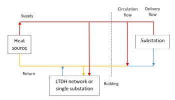
Figure 94. General layout for the return-to-return variant of the Warm – Classic configuration
