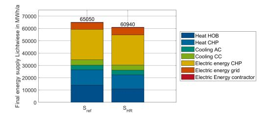
Figure 63. Impact of the proposed temperature reduction measures on final energy supply.
