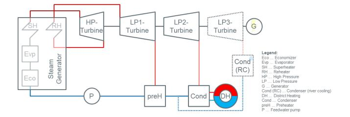
Figure 13. Visualisation of the combined heat and power generation (CHP) model and its main components. The components represented using solid lines represent the back-pressure turbine. The additional components on the right (dotted lines) represent the extraction-condensing turbine. More electricity is generated per unit of heat in combined heat and power plants because higher power-to-heat ratios are obtained by lower steam pressures in the turbine condensers.
