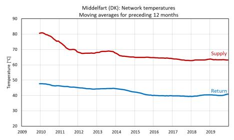
Figure 38. Supply and return temperatures for the Middelfart (DK) district heating network (Middelfart Fjernvarme, 2020).
