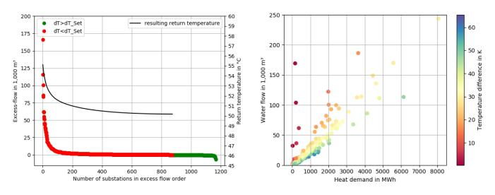
Figure 33. The excess flow analysis approach allows analysis and visualisation of the reduction potential of return temperature in existing district heating networks (left: ranking of substations according to their current impact on the return temperature of the district heating network; right: water flow linked with heat supply).
