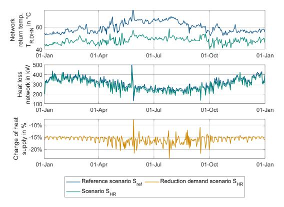
Figure 62. Impact of the proposed temperature reduction measures on network return temperatures, heat losses, and heat supply.
