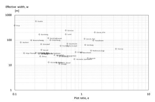
Figure 70. Effective width as a function of the plot ratio.
