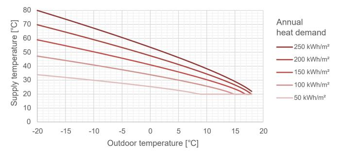
Figure 25. Example of supply temperatures required in a radiator system when various levels of energy renovation are carried out in a building.
