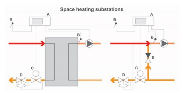
Figure 22. Example of the basic layout for an indirect (left) and a direct (right) space heating substation. (A) Controller, (B) Temperature sensors, (C) Actuator and control valve, (D) Differential pressure controller, and (E) Non-return valve.
