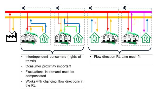
Figure 41. Options for direct or indirect cascading connection of high- and low-temperature customers: a) direct use of a high-temperature return; b) double cascade, the indirect use of a high-temperature customer and direct use with admixture; c) indirect use of the high-temperature return via the return pipe of the heating network; and d) indirect use via the supply pipe of the district heating network (Köfinger et al., 2016)
