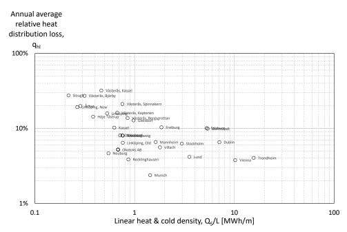
Figure 72. Relative annual heat distribution loss as a function of the linear heat density.
