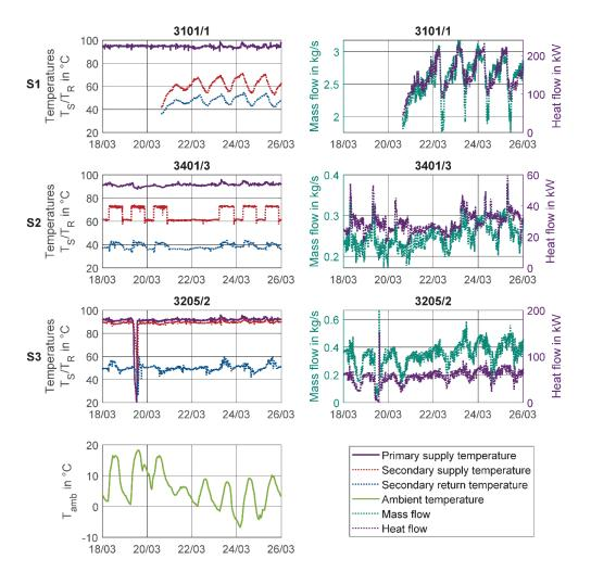
Figure 57. Temperatures, mass flow, and heat flow for the three categories S1-S3 of well-functioning space heating circuits
