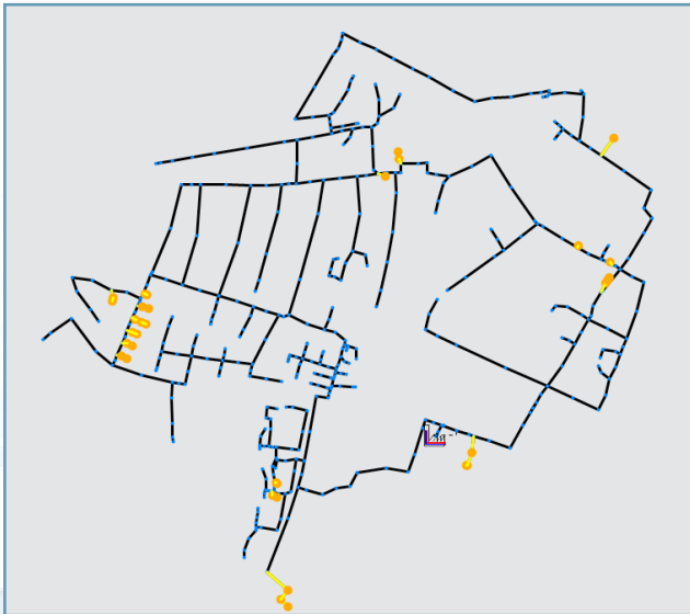
Figure 4-9 Original network and removed street pipes (Lund et al. 2014, Brand 2013, Yang 2016 and Bartram et al. 2007).
